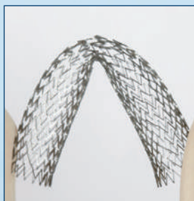
Competitors: laser cut nitinol stent made from the tube
